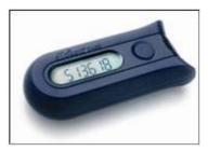
• **eToken NG-OTP:** An integrated hybrid USB smartcard and OTP token. The authenticators operate as either a smartcard when attached to a PC using the USB connector or as an OTP token when detached.
