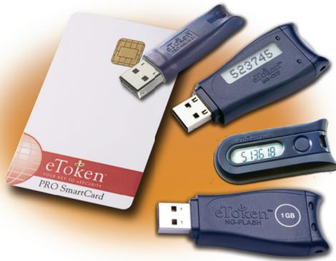
The Aladdin eToken devices run on the Java card operating system, which enables multiple applications to be deployed on a single smart card, and new ones to be added even after the token has been issued to the end user. Java card technology also makes it easy to integrate security tokens into a complete Java software solution.
